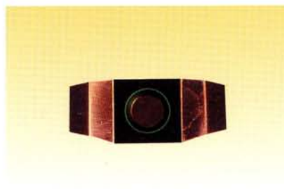
EIAJ ET-7404 compatible copper plate for rapid heating
