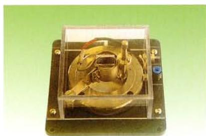
Preheating device and N 2 chamber
