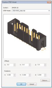
Position STEP Models in a footprint using the graphical dialog
