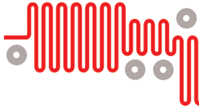
Complex serpentine routing can be easily defined and constructed
