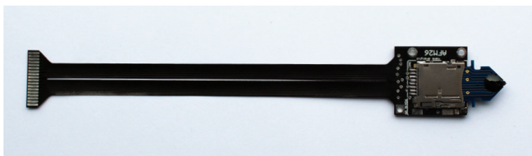
Cantilever holder with integrated first-stage amplifier and flat-cable: Type AFM 26 (120mm length) Type AFM 27 (90mm length) PCB dimensions (mm) 23 x 22
