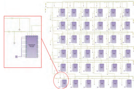
An RC delay circuit to the mirror actuating electrodes
