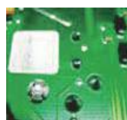
PIN foot welding
