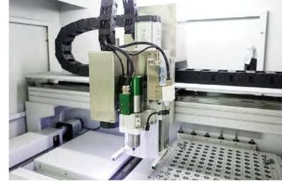
1. The feeding arm is modular design, which can helps fast line changing and improve line changing efficiency up to 50%. Compared with the single gripper, the dual grippers can let the loading and unloading
