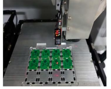
4、Barcode camera can dynamically capture and identify QR codes at any position. Pratical application QR code: min2.5\*2.5mm(Optional)
