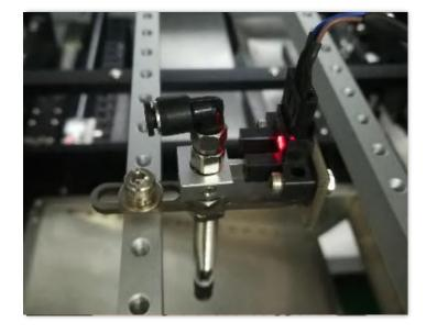
Simple functional device, by adjusting the position of the sensor on the nozzle rod to match the buffer nozzle, when the PCB panel is placed, it will trigger the sensor alarm when there are foreign objects or the higher parts on the back touch the fixture. To Protect the substrate..
