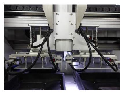
6. Gripper module is suitable for no edge cutting technology, fixture in and out and pick up large and heavy PCBA (Optinal)
