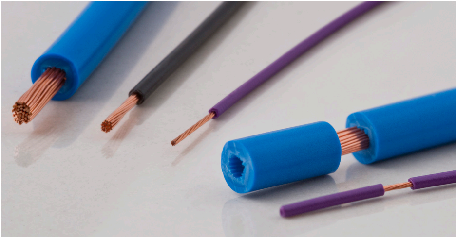
▲ Processing samples Conductors with full and partial pull-off
