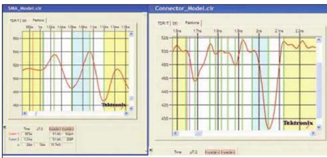
FIGURE 6. Modeling of SMA (left) and the connector-via reflections region (right) by partitioning the impedance profile of the respective regions.
