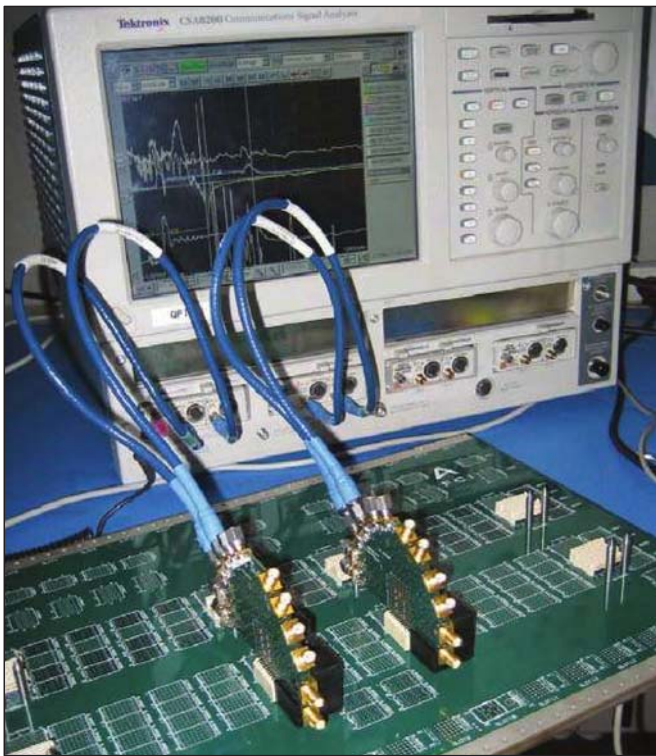
FIGURE 4. Measurement setup for backplane measurements. The test cards are connected to Module 6 Slots 7 and 10. The Tx trace is K&L6 and Rx trace is E&F6.
