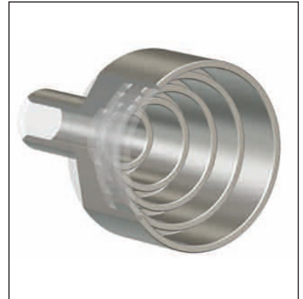
▲ Fig. 5 Horn antenna with reflective metallic surface.
